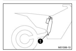
The shock absorber article number **1** is stamped on the base of the shock absorber.
