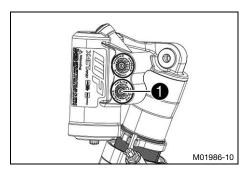
Turn adjusting screw 1 clockwise with a hexagon socket wrench up to the last perceptible click.
