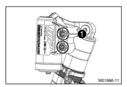
Turn adjusting screw 1 clockwise with a hexagon socket wrench up to the last perceptible click.
